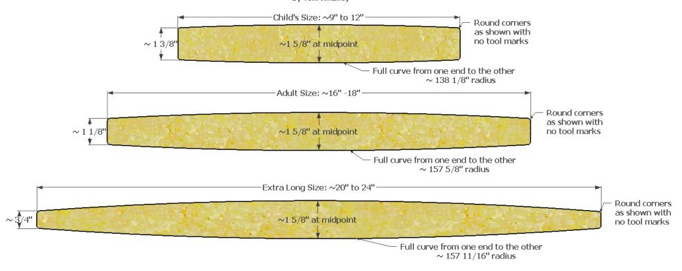
Actual curvature of the Rolling Pins - attach to 3/4" thick piece of wood to cut out for a sanding block
