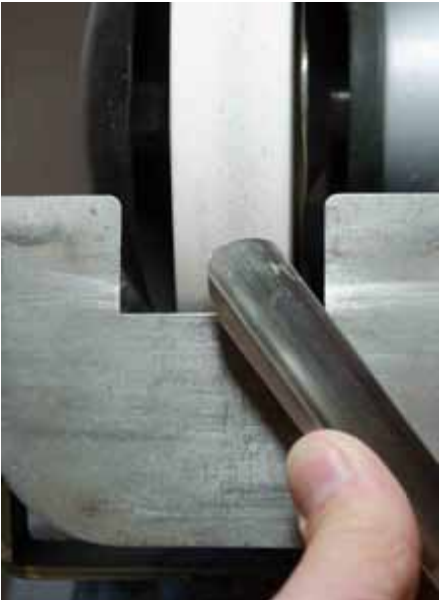
4 Sharpening. Swing the handle right while rotating the flute.
