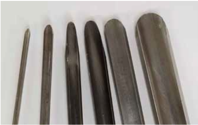
1 Spindle gouges. The fingernail shape is typical, with a finer, more pointed tip for detail work.
