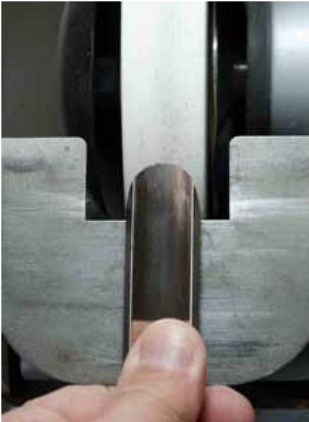
3 Sharpening. Start in the center with the flute facing up.
