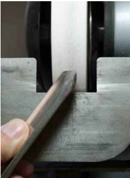
5 Sharpening. Swing left while rotating the flute.
