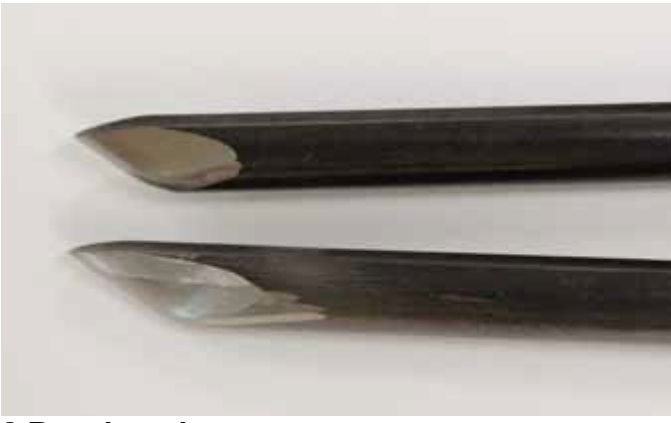
2 Bevel angle. Top, 35° bevel, with rounded heel. Bottom, short 35° bevel with three secondary bevels.
