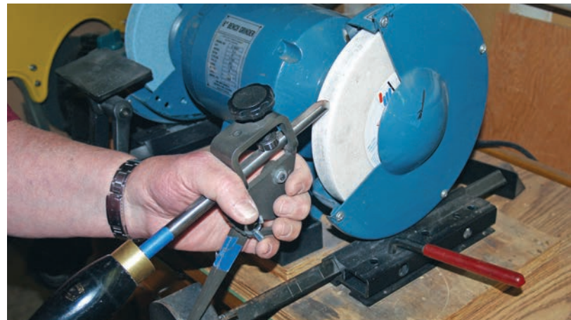
Wrong way! If the sharpening jig slips, fingers will contact the rotating wheel before the jig does.
