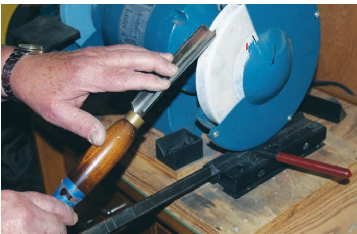
Better: Create a more acute bevel angle on your tool, which will place it higher up on the wheel in a safer position when sharpening.
