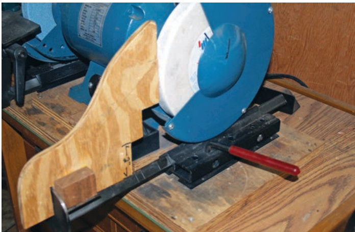
Using a simple shopmade template to set up your sharpening jig for repeatable distances saves time and tool wear.
