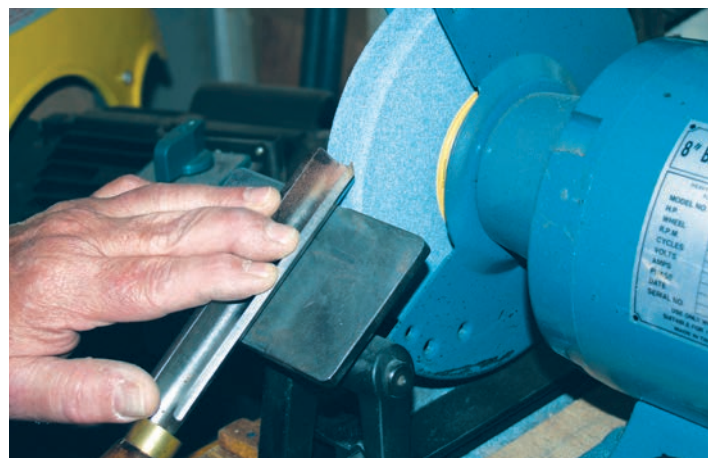
Consider learning how to hand sharpen turning tools. This allows you to place a toolrest close to the grinding wheel, eliminating many potential dangers.
