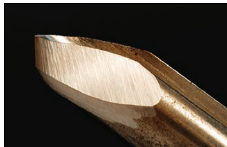
This 3/8" bowl gouge has a fingernail grind.
