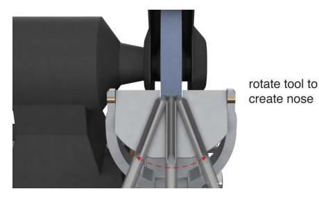
To grind the nose of the gouge, twist and swing at the same time.
