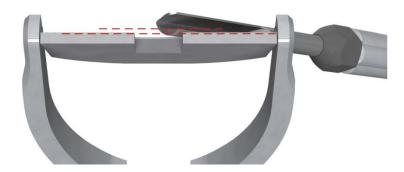
When grinding the wing, the flute should be slightly open, so that the inside wall of the wing is parallel with the surface of the platform.
