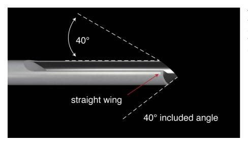
The 4o/40 bowl gouge gets its name from the grind, which produces a 40 degree bevel on the nose and wings of the gouge, with straight wings which are swept back at a 40 degree angle.
