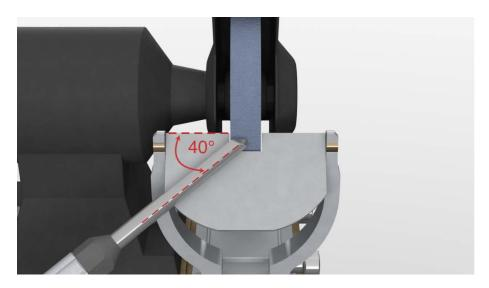
In order to create the 40 degree swept back wings, place the tool on the platform at 40 degrees from horizontal.
