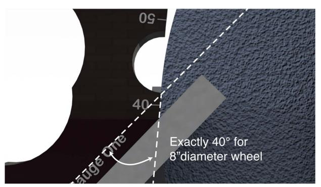
To set up the grinder platform, make sure that there is a 40 degree angle where it contacts the wheel.
