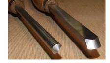
made. When the bevel does not rub the wood as the cut is being made, the gouge edge becomes like a scraper and actually tears the wood fibers, as well as making the whole cut rather unstable. However, scraping cuts (and scrapers!) definitely have their place.
