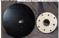
it to allow screws to pass through and into the base of the wood. This is the oldest and perhaps still most common way of holding bowl blanks and other large pieces of wood safely and effectively. As long as one remembers to account for the depth of the screws and not hollow down to them, the workpiece and be held very securely.
