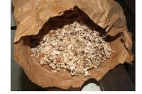
Green wood will warp as it dries, and therefore many turners who want to turn wood while green (and therefore usually more soft) will rough turn a piece and then store it in a controlled environment to minimize wood movement (see photo). Once dried, the wood will be re-turned and finished as desired, sometimes 6 months or more after initial green turning.
