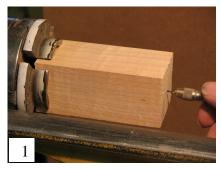
Prepare 4" long blank, 1-3/4" square and mount in chuck as pictured above. Drill 1/16" pilot hole in end of blank for later installation of screw eye for dying.
