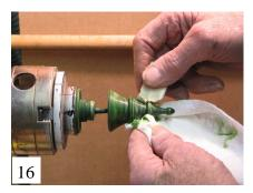
After dry polish, apply Hut Perfect Pen polish stick wax to surface, again applying pressure on opposite side with towel. After application of Hut stick wax, polish as with previous photo #15.
