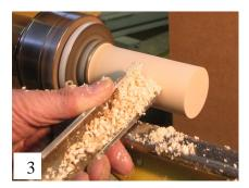
Turn blank end to end and remount with tennon in chuck. Finish turning to a uniform 1-5/8" diameter.
