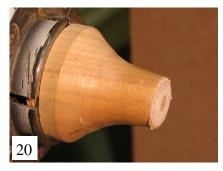
Turn a fixture with about 1" diameter on outer end. Shape the face a little convex. Attach 120 grit sticky sand paper (or glue your own) to the face.
