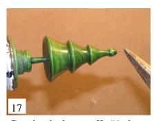
Cut hook loop off #1 long shank fish hook leaving straight shank with eye in one end. Using pliers, push shank in rotating ornament stopping 3/16" from bottom. Stop lathe and tap to bottom like a nail.
