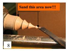
Use long point of skew to cut a dimple into end of ornament for centering hanger eye later. Do <u>all</u> sanding thru final 400 grit between points before next step. If you sand AFTER tree trunk is cut, you will break it.
