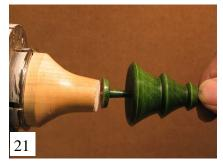
Sanding base of tree. In photo #11 I had directed you to establish the base with a 1/16" deep cut. This shallow cut prevented dye from penetrating bottom of ornament. This left clean area to sign & date.
