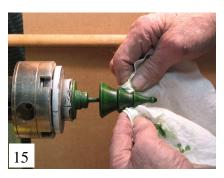
Air dry 5 to 10 minutes then remount into chuck. Run lathe at slow speed, us Viva paper towel & polish entire surface exerting EQUAL pressure on EACH side of ornament to prevent bending & breaking.
