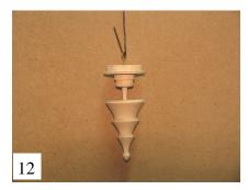
Do not part off base at this time. Remove from lathe, install small eye screw in bottom pilot hole and hang from 12" long piece of straight stiff wire with tight hook.
