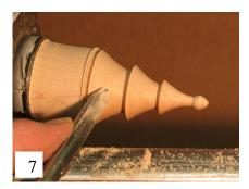
Use spindle gouge to make sweeping cuts from left to right on each segment swinging the tool handle through an arc to make each segment a curved section. Shape oval ball at tree tip.
