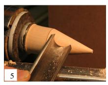
Use spindle roughing gouge to cut uniform 'cone' shape from mark on blank to a diameter of about 3/16" on right end of 'cone'.
